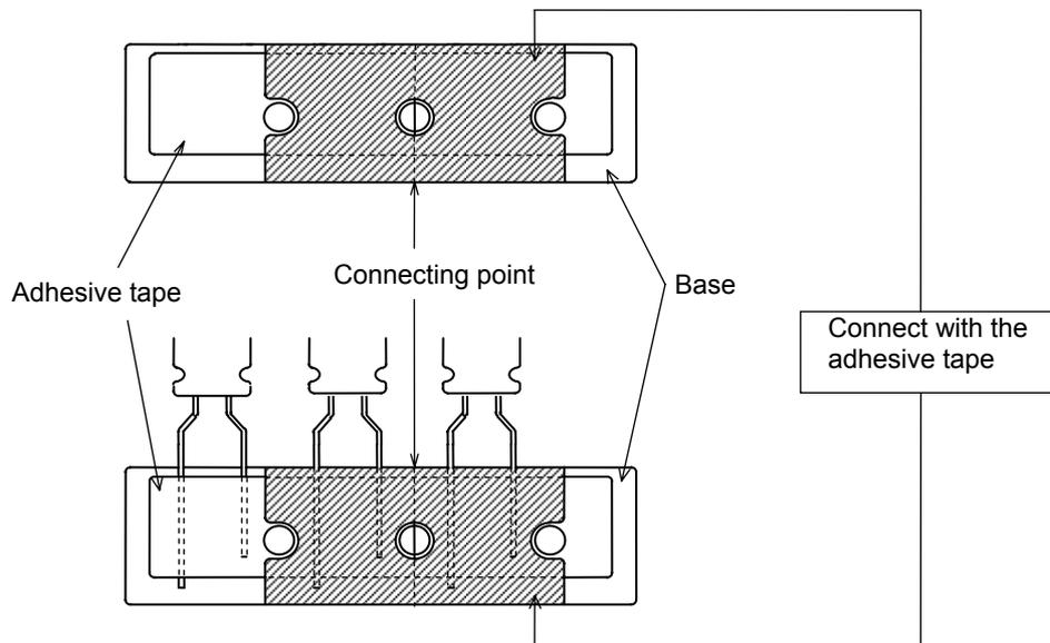
Note ) When connecting two base tapes, they shall not be piled on top of each other. Base tapes shall not be connected with each other by using staples.
