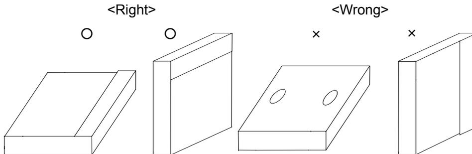
12-4 The inner cartons shall be packed in a cardboard box for transportation. Products with various part numbers can be packed in an outer carton upon request. However, each inner carton (the smallest packing unit) shall only contain products with the same part number.
