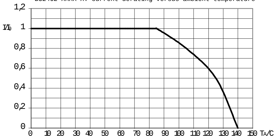
B82462-XXXX-X: current derating versus ambient temperature
