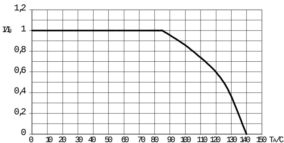
B82464-XXXX-X: current derating versus ambient temperature
