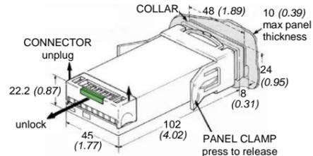
Optional panel adaptors are available for the controllers to be mounted in a 45x45mm (1/16DIN) cutout.
