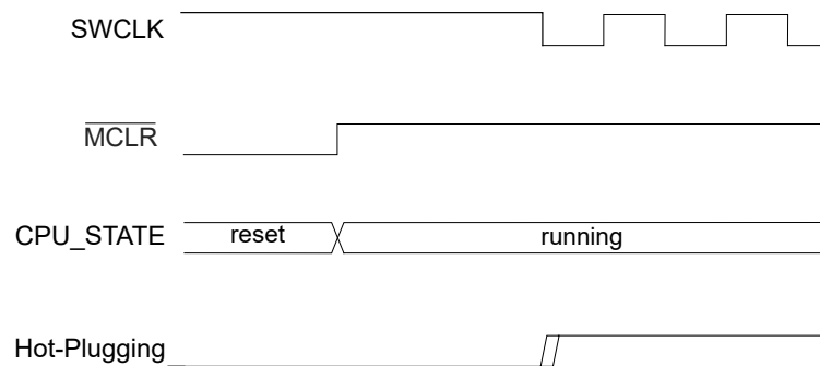
Figure 17-3. Hot-Plugging Detection Timing Diagram
