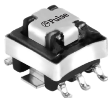
Part 6,7 Number Turns Ratio Current 2 Rating (A) Secondary Inductance (mH MIN) DCR (mΩ MAX) Hipot (V RMS ) Primary (8-7) Secondary (1-3) P8202NL 1:20 10 0.08 6 550 500 P8203NL 1:30 10 0.18 6 870 500 P8204NL 1:40 10 0.32 6 1140 500 P8205NL 1:50 10 0.50 6 1500 500 P8206NL 1:60 10 0.72 6 2250 500 P8207NL 1:70 10 0.98 6 4700 500 P8208NL 1:100 10 2.00 6 6000 500 P8209NL 1:125 10 3.00 6 6500 500
