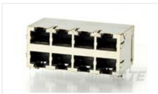
TE Part #5569257-1 STK MJ ASSY, 8POS, 2X4, SHLD, CAT5
