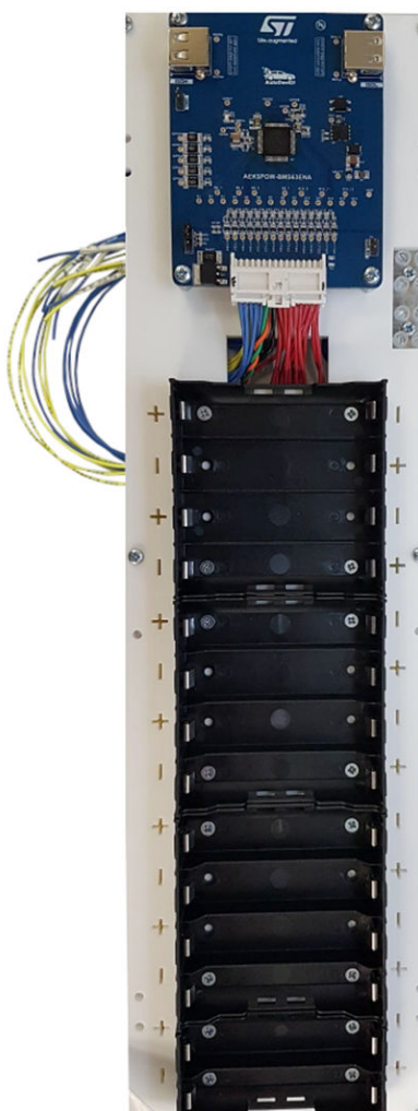
Figure 4. Cables to connect external NTCs
