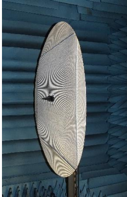
antenna sample measured on \varnothing 52\text{in} (1.3m) ground plane
