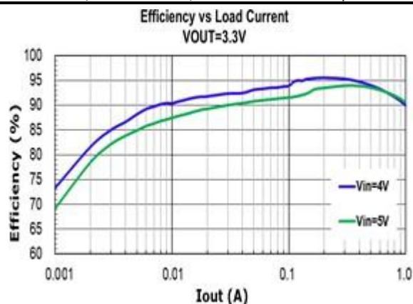
FIG.33 EFFICIENCY V.S. LOAD CURRENT
