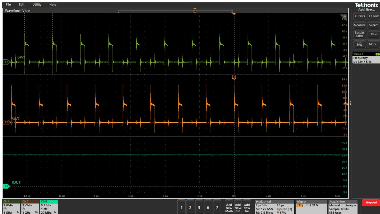
Figure 22 Switch node waveforms at 25A
