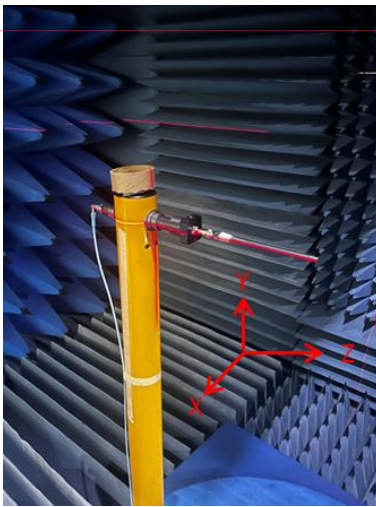
Chamber Set-up in Free Space.
