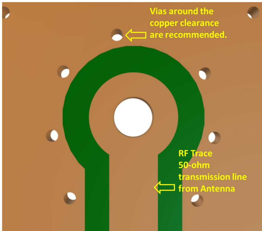
Bottom view of the PCB Reference Design, showing transmission lines and integration notes.
