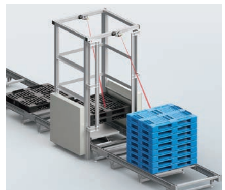
Detecting how many pallets are remaining
