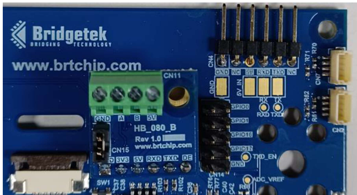
Figure 8 – IDM-RS485 Daughter Board Mounting Orientation
