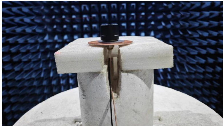
Radiation element is test on D120mm ground plane
