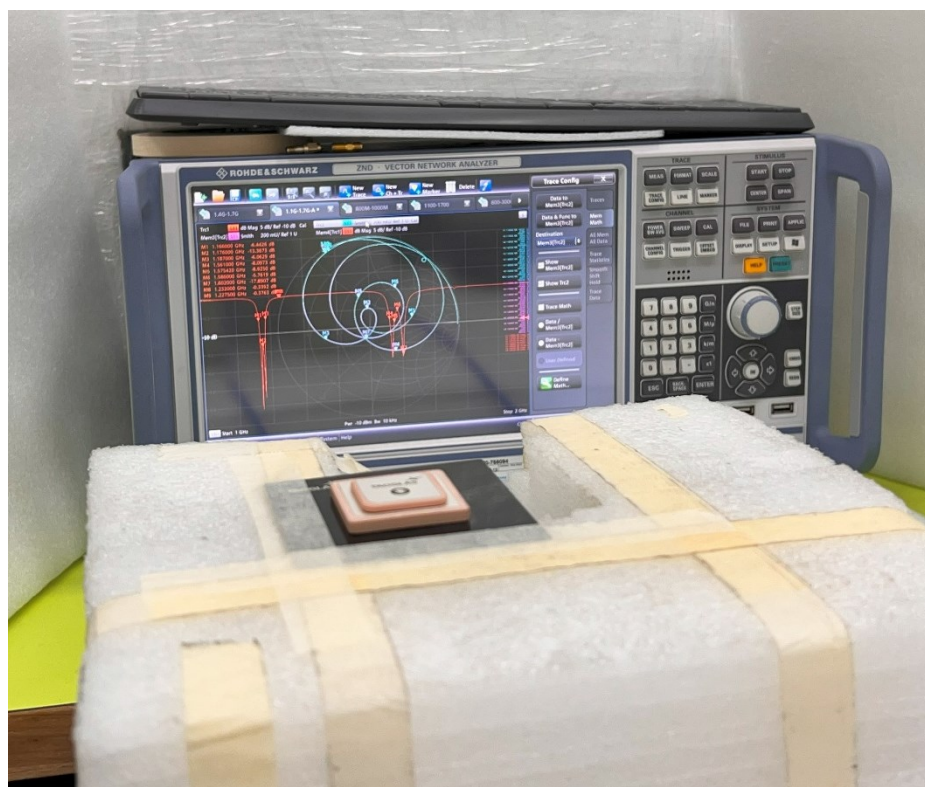
VNA Test Setup on a 70 x 70mm Ground Plane
