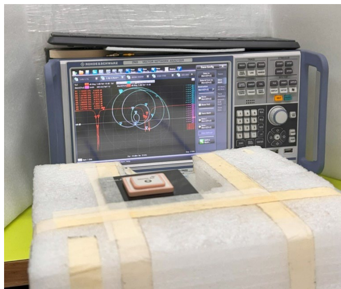
VNA Test Setup on 70x70mm Ground Plane
