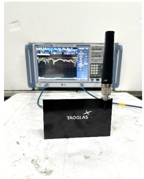
VNA Test Set-up – 15x9cm Ground Plane
