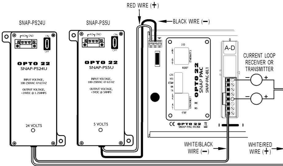
**Figure 2. SNAP-PS24U Used as a Loop Supply with Legacy Hardware**
