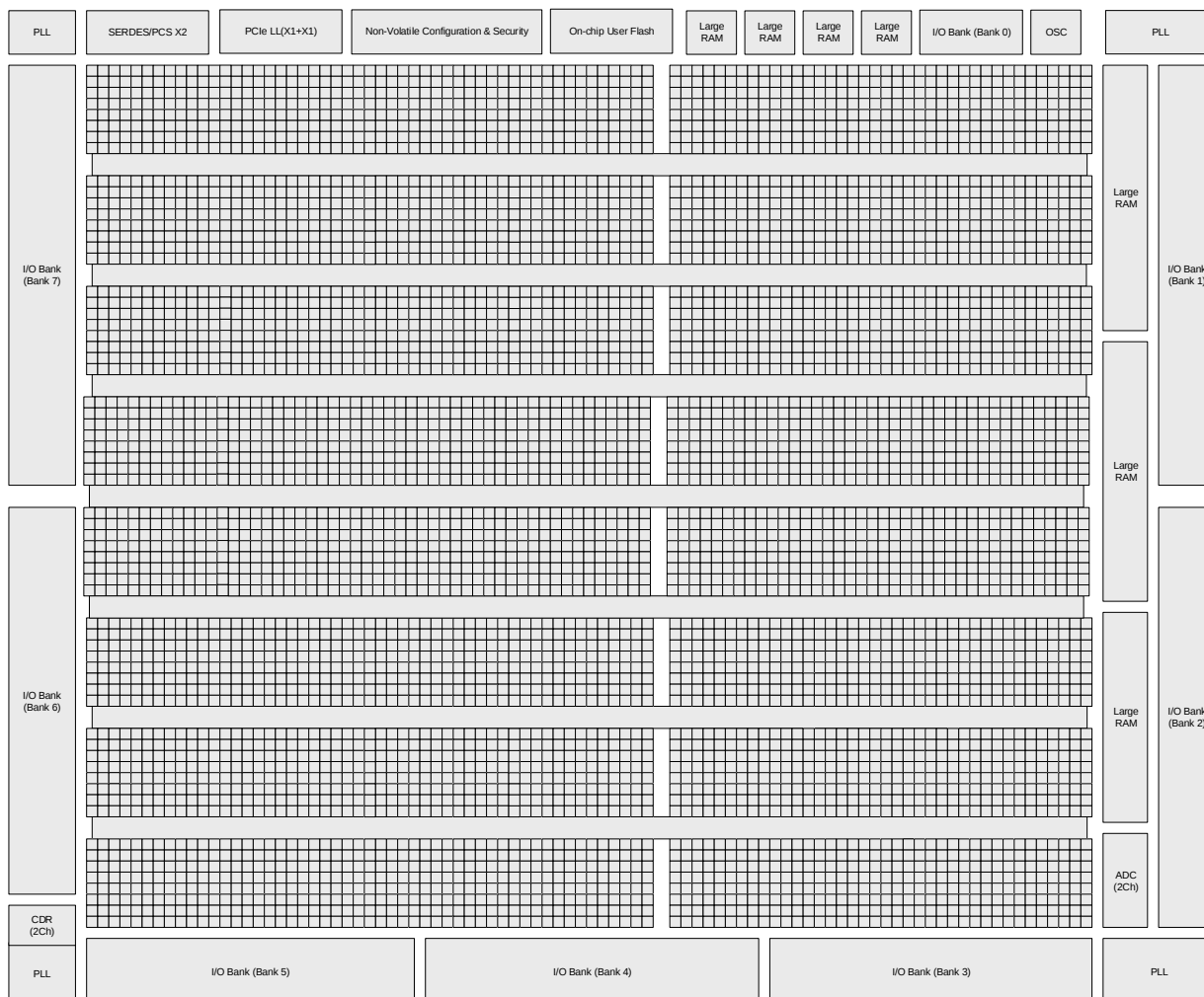
Figure 2.3. Simplified Block Diagram, MachXO5-NX-100T Device (Top Level)
