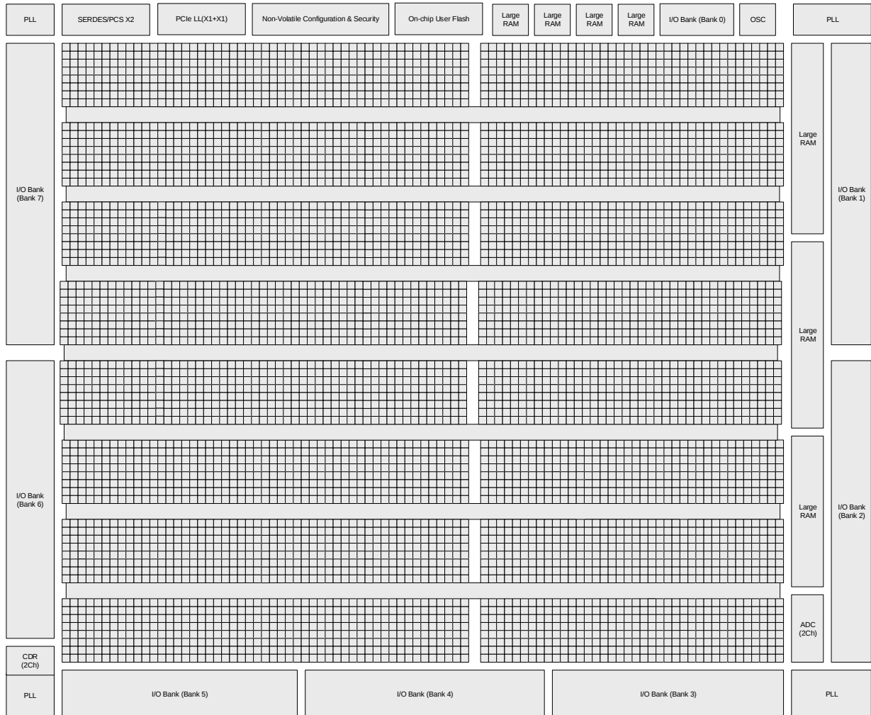
Figure 2.2. Simplified Block Diagram, MachXO5-NX-55T Device (Top Level)
