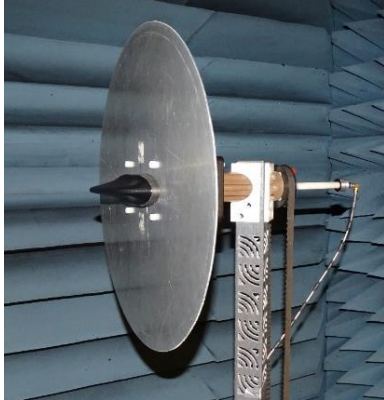
antenna sample measured on Ø24" (609.6mm) ground plane
