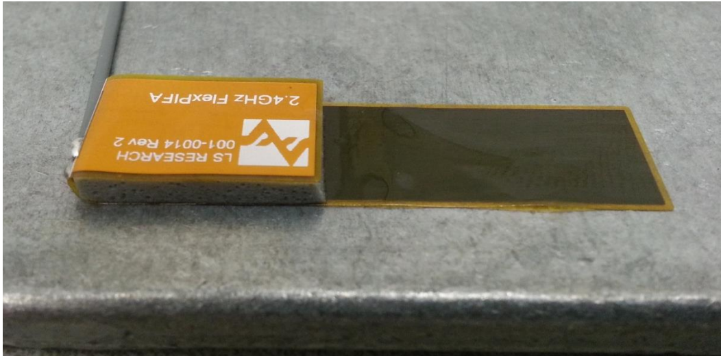
Figure 25: FlexPIFA mounted on metal
