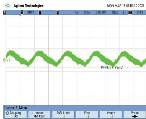
Ripple & Noise PQU1000-48; Full Load; 264Vac Input
