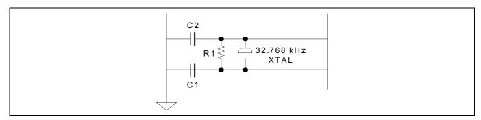
Figure 2 32 kHz oscillator block diagram
