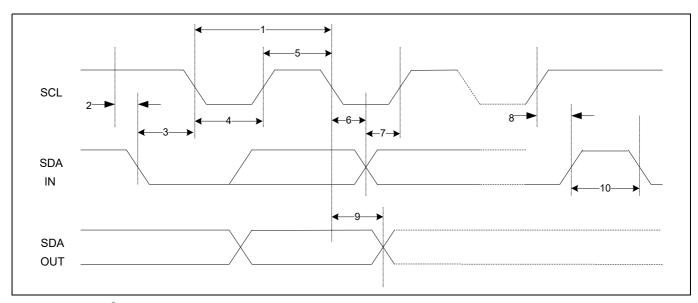
Figure 14 I<sup>2</sup>C interface timing diagram
