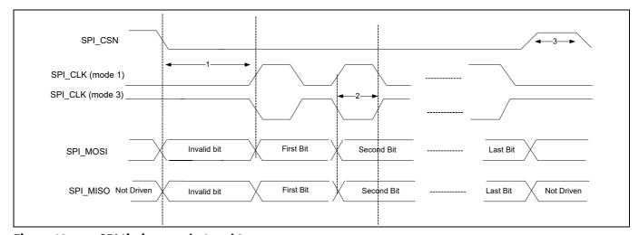
Figure 13 SPI timing, mode 1 and 3
