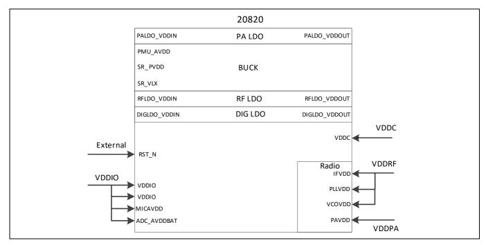
Figure 7 Configuration 2 - External supplies
