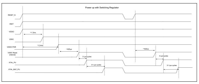
Figure 4 Reset timing
