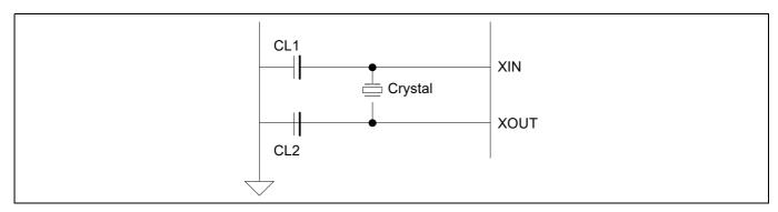
Figure 1 Recommended oscillator configuration
