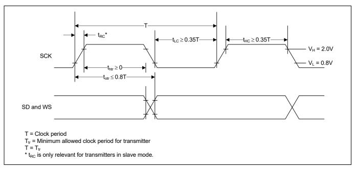
Figure 15 I<sup>2</sup>S transmitter timing
