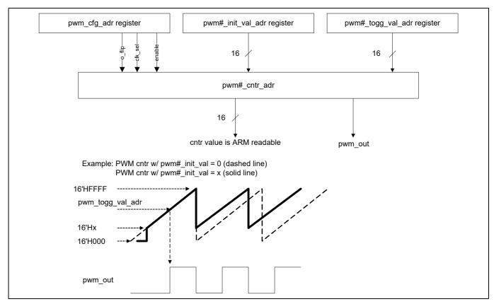
Figure 9 PWM block diagram
