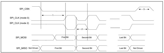
Figure 12 SPI timing, mode 0 and 2
