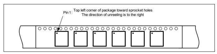
Figure 18 Pin 1 orientation
