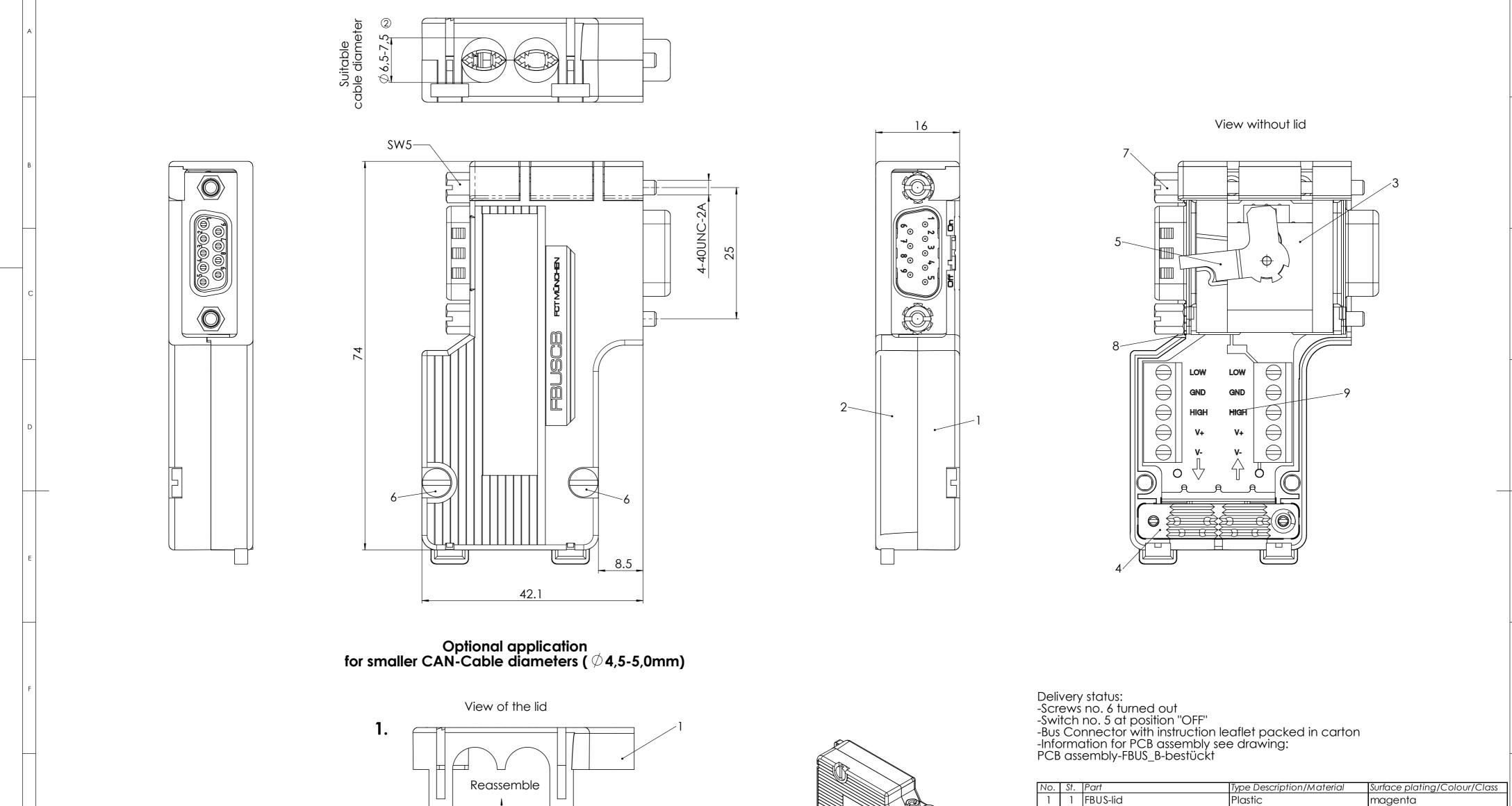
For CAN- cable diameters of ø4,5-5,0mm the strain relief in the lid must be dismantled by srew driver and reassembled again with the strain relief turned by 180° with the springs dismantled.
