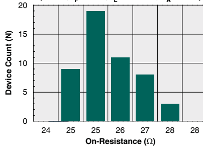
Typical On-Resistance Distribution (N=50, I_F=0\text{mA} , I_L=100\text{mA} , T_A=25^\circ\text{C} )
