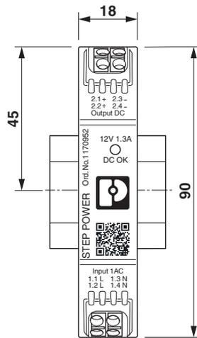
Figure 6 Device dimensions (dimensions in mm)
