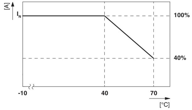
13.3.4 Rotated mounting position 270° Z-axis
