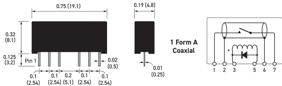
**Important:** Where the optional internal diode is fitted or for all Form B types, the correct coil polarity must be observed, as shown by the + symbol on the schematics.
