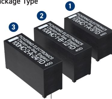
The Series 100HC Form A versions offer higher coil resistances than the similar specification Series 114, the greater winding space allowing for the use of switches rated to 3 Amps continuous carry current and even higher levels in pulsed current applications.
