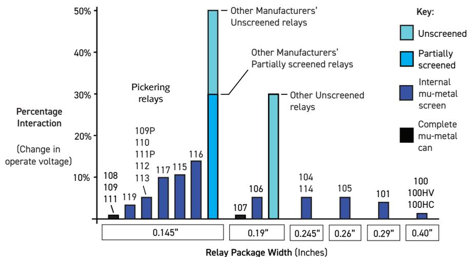
This chart demonstrates the percentage changes in operate voltage due to magnetic interaction depending on the level of magnetic screening offered from the relay package. For more information on magnetic interaction [click here](#).
