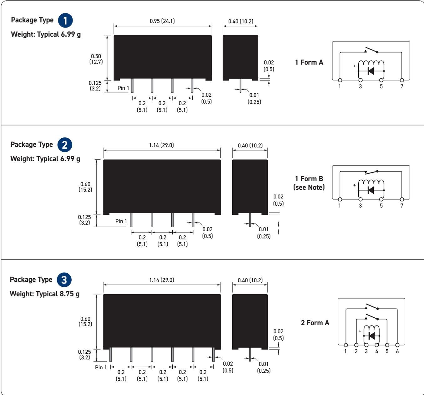
**Important:** Where the optional internal diode is fitted or for all Form B types, the correct coil polarity must be observed, as shown by the + symbol on the schematics.
