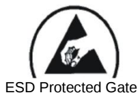
ESD Protected Gate
