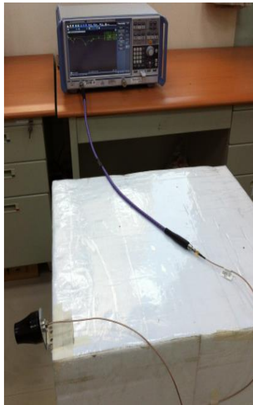
Figure1. Measurement Setup of G30 Antenna in Free Space, 30cmx30cm metal plate and L-shaped frame.
