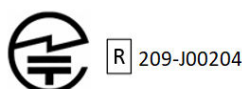
Figure 11.2. Compliance Mark with Certification Number to be Placed on the Outside Surface of the Host Equipment
