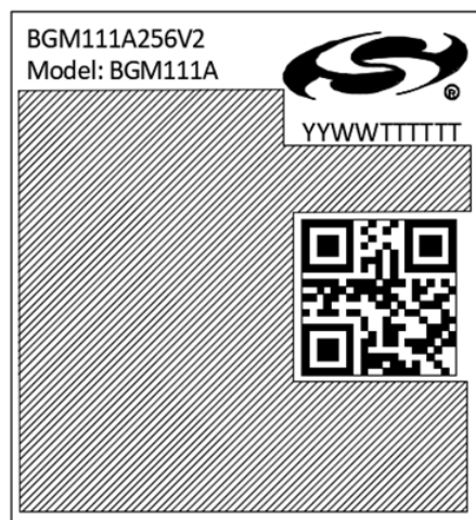
Figure 8.3. BGM111 Package Marking
