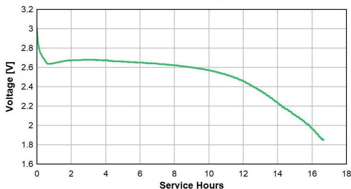
Pulse Discharge 10mA 5s/m, 24hd until 1.8V
