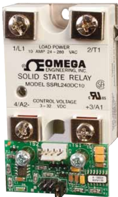
PCM4 shown actual size mounted on SSR240DC10
