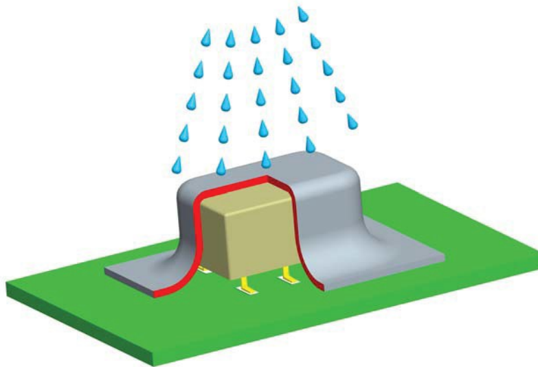
Fig. 4: Coating of relays on PCB's
