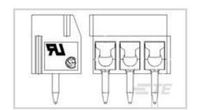
Terminal Block Connector Type: Header
