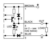
NOTE: in case of combined load, i.e. resistive and capacitive, the maximum admissible capacity (C) is  $1\mu\text{F}$  for maximum output voltage and current.
