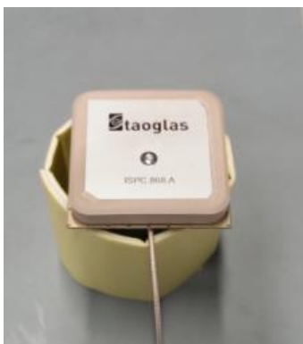
Ground under antenna
