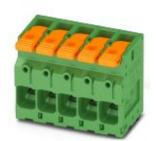
PCB terminal block, nominal current: 76 A, rated voltage (III/2): 1000 V, nominal cross section: 16 mm², Number of potentials: 6, Number of rows: 1, Number of positions per row: 6, product range: LPT 16/, pitch: 10 mm, connection method: Lever Push-in connection, mounting: Wave soldering, conductor/PCB connection direction: 0 °, color: green, Pin layout: Zigzag pinning W, Solder pin [P]: 3.6 mm, type of packaging: packed in
