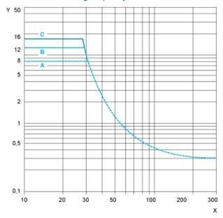
(y) Current DC (x) Voltage DC A: RSB2A080 •• B: RSB1A160 •• C: RSB1A120 ••
