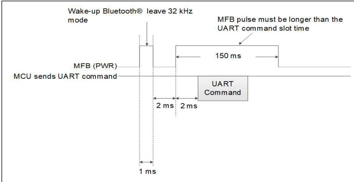
**FIGURE 5-5: TIMING SEQUENCE OF POWER-OFF STATE**
