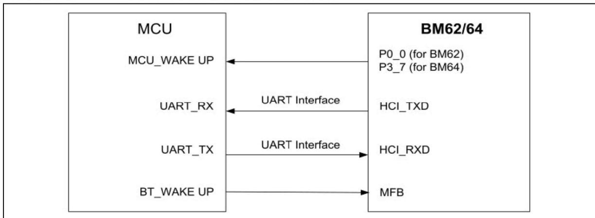
An external MCU can control the BM62/64 module over the UART interface and wake-up the module with the MFB, P0\_0 (BM62) and P3\_7 (BM64) pins.
