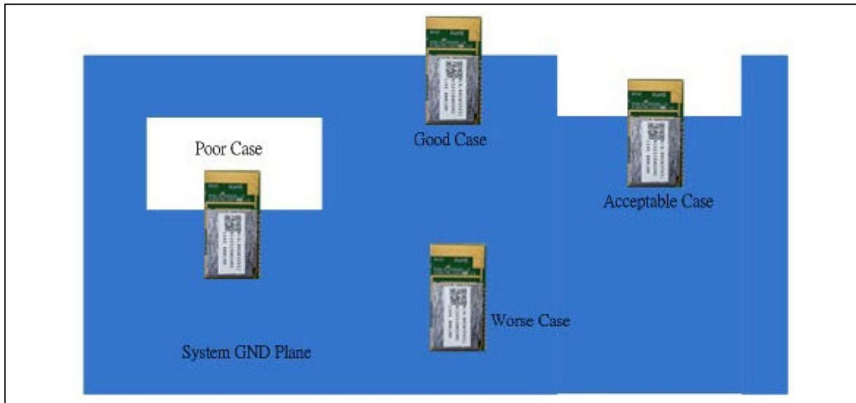
**FIGURE 6-4: GND PLANE ON MAIN APPLICATION BOARD**
