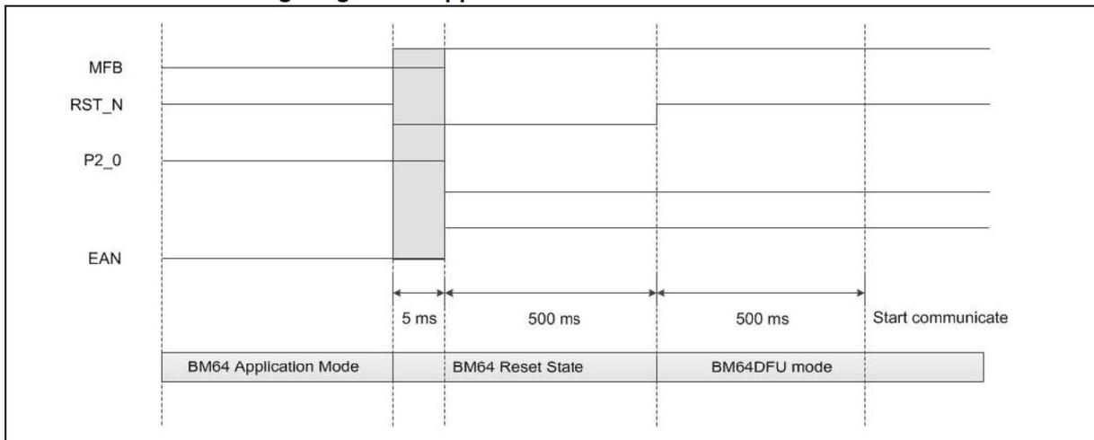
Be sure to switch back from “ROM TEST/DFU” mode to Application mode, after the DFU, as illustrated in following figure.
