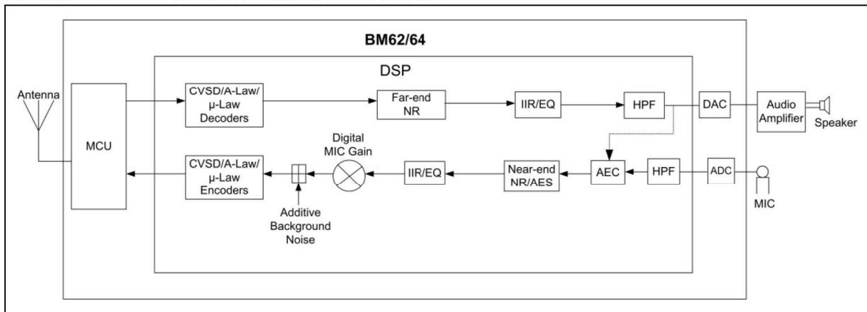
**FIGURE 2-2: AUDIO SIGNAL PROCESSING**
