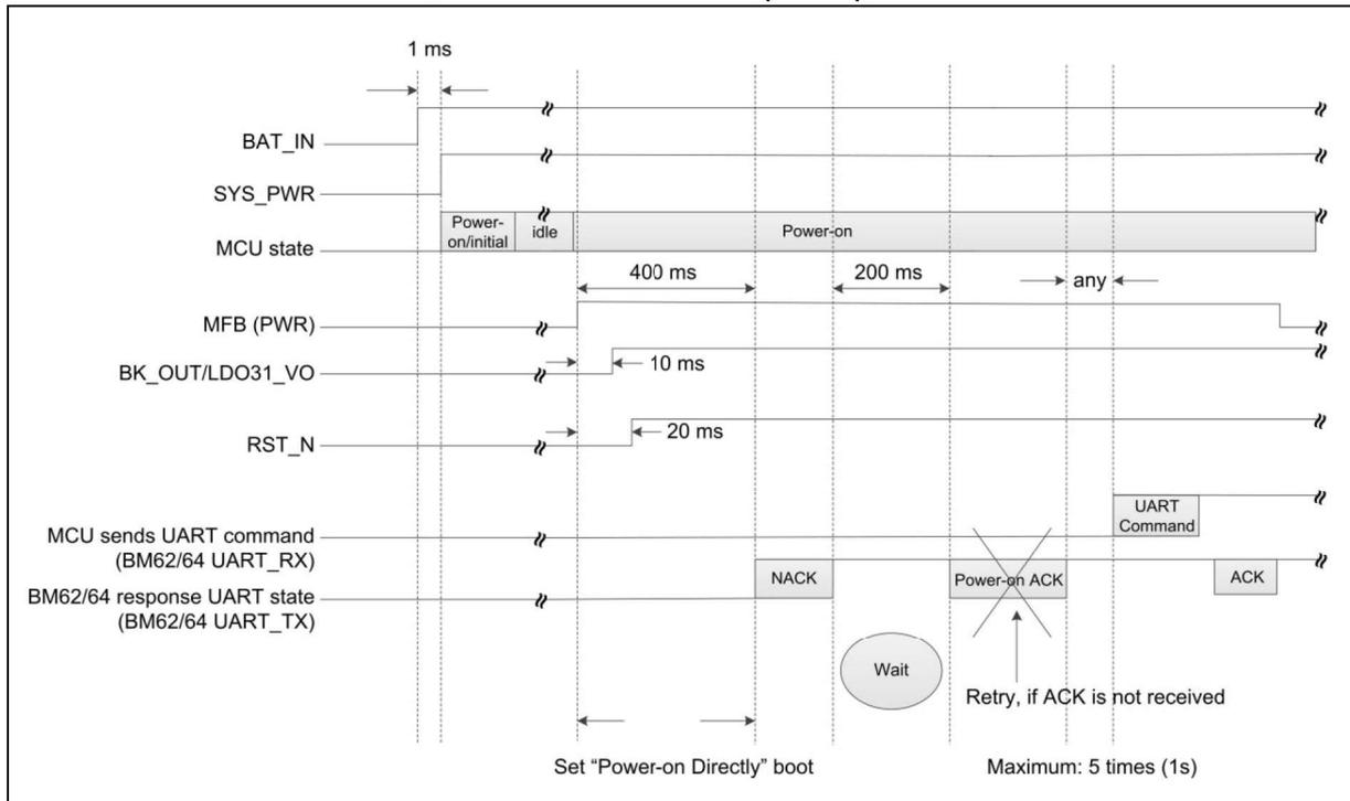
**FIGURE 5-7: RESET TIMING SEQUENCE IN NO RESPONSE FROM MODULE TO HOST MCU**
