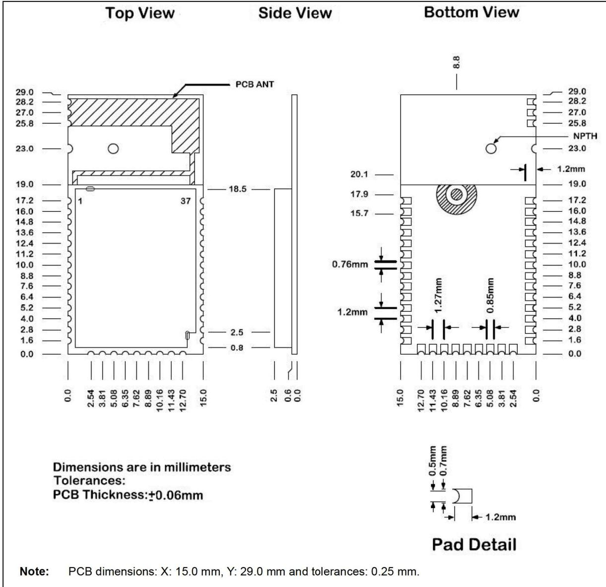
Figure 7-2 illustrates the PCB dimension of the BM64 module.
