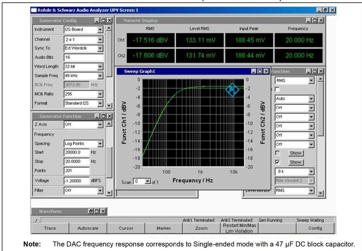
**Note:** The DAC frequency response corresponds to Single-ended mode with a 47  $\mu$ F DC block capacitor.
