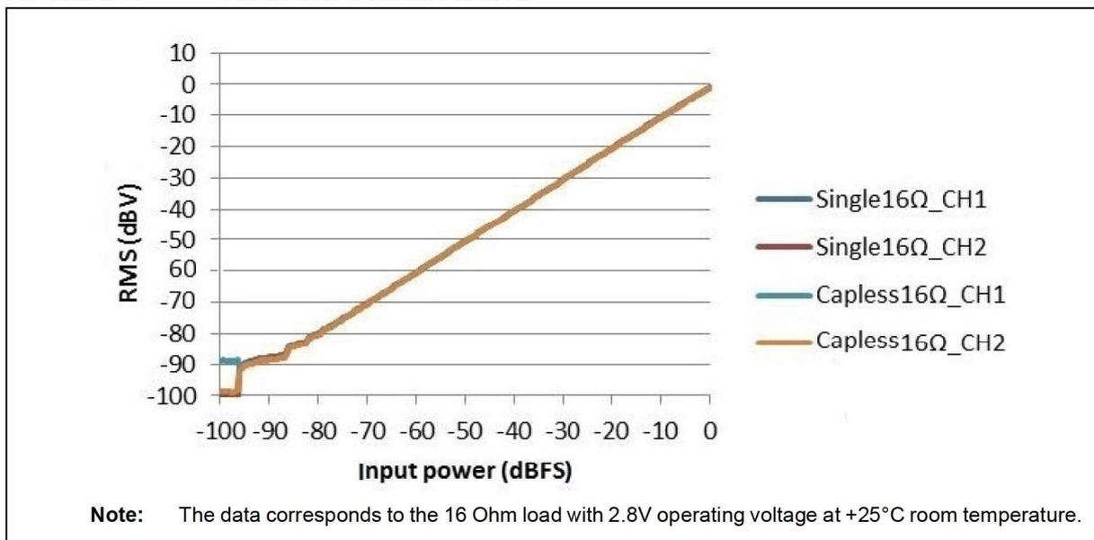
FIGURE 2-4: CODEC DAC THD+N VERSUS INPUT POWER
