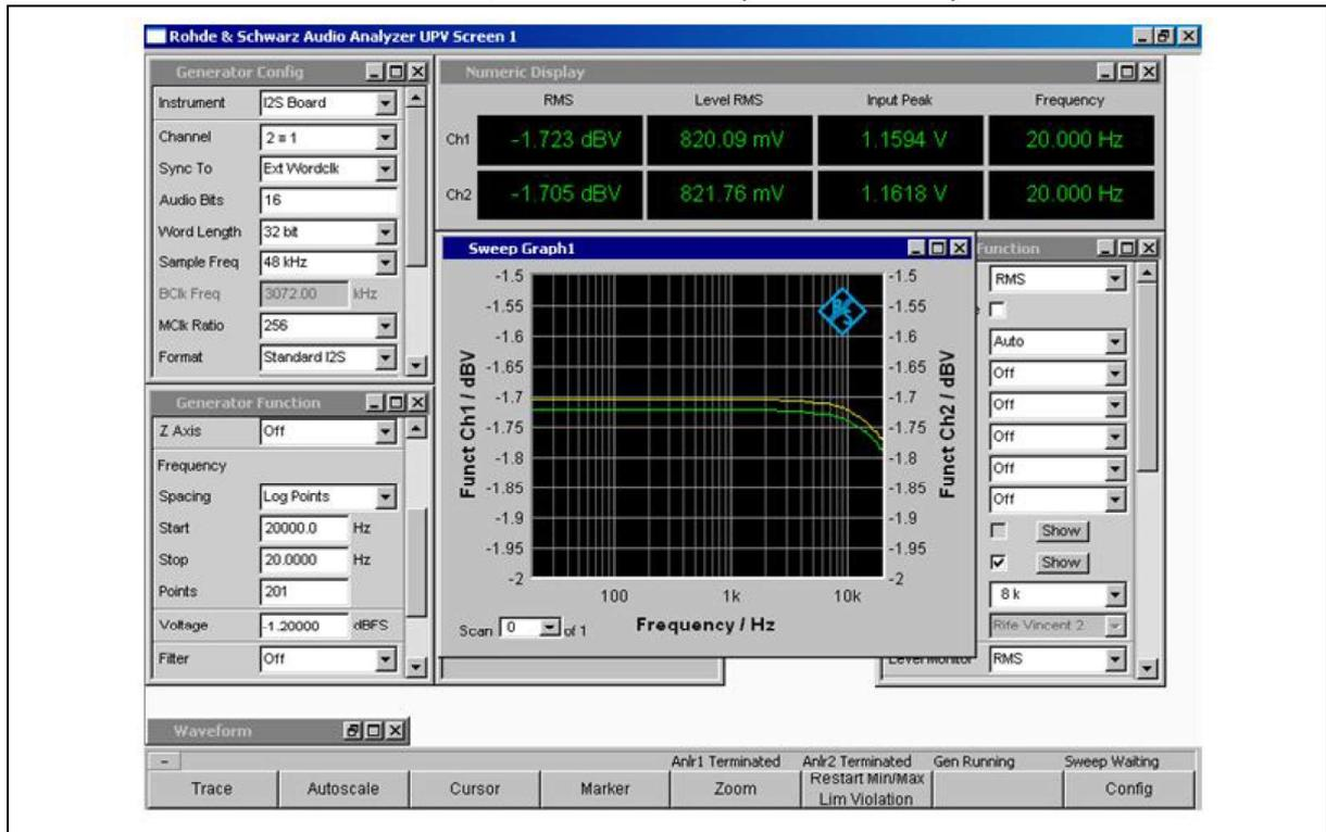
**FIGURE 2-6: CODEC DAC FREQUENCY RESPONSE (SINGLE-ENDED MODE)**
