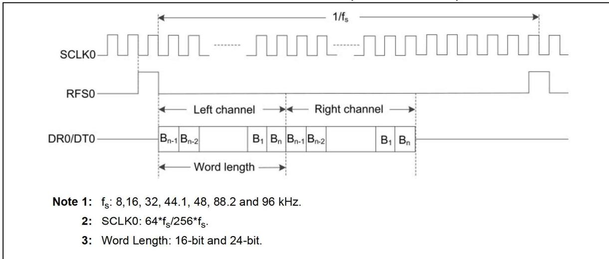
Figure 8-3 illustrates the timing diagram of the audio interface.
