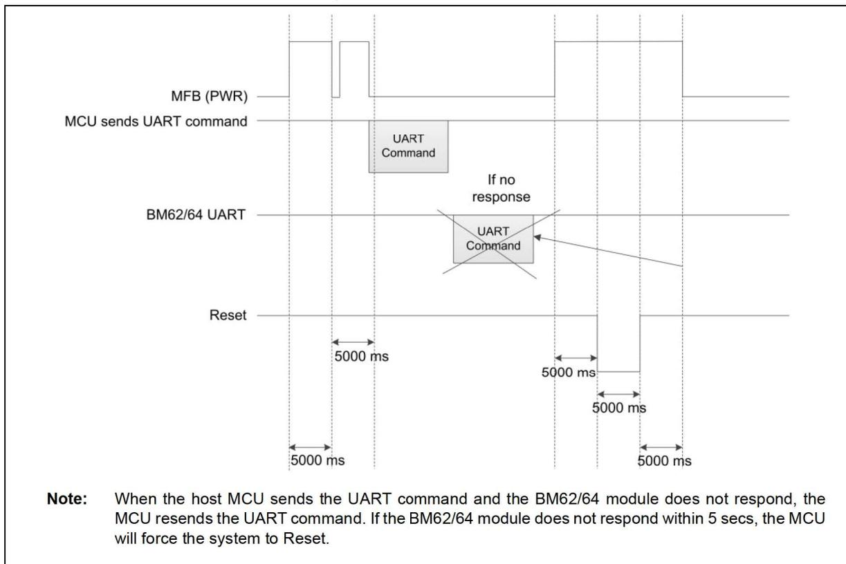
**Note:** When the host MCU sends the UART command and the BM62/64 module does not respond, the MCU resends the UART command. If the BM62/64 module does not respond within 5 secs, the MCU will force the system to Reset.
