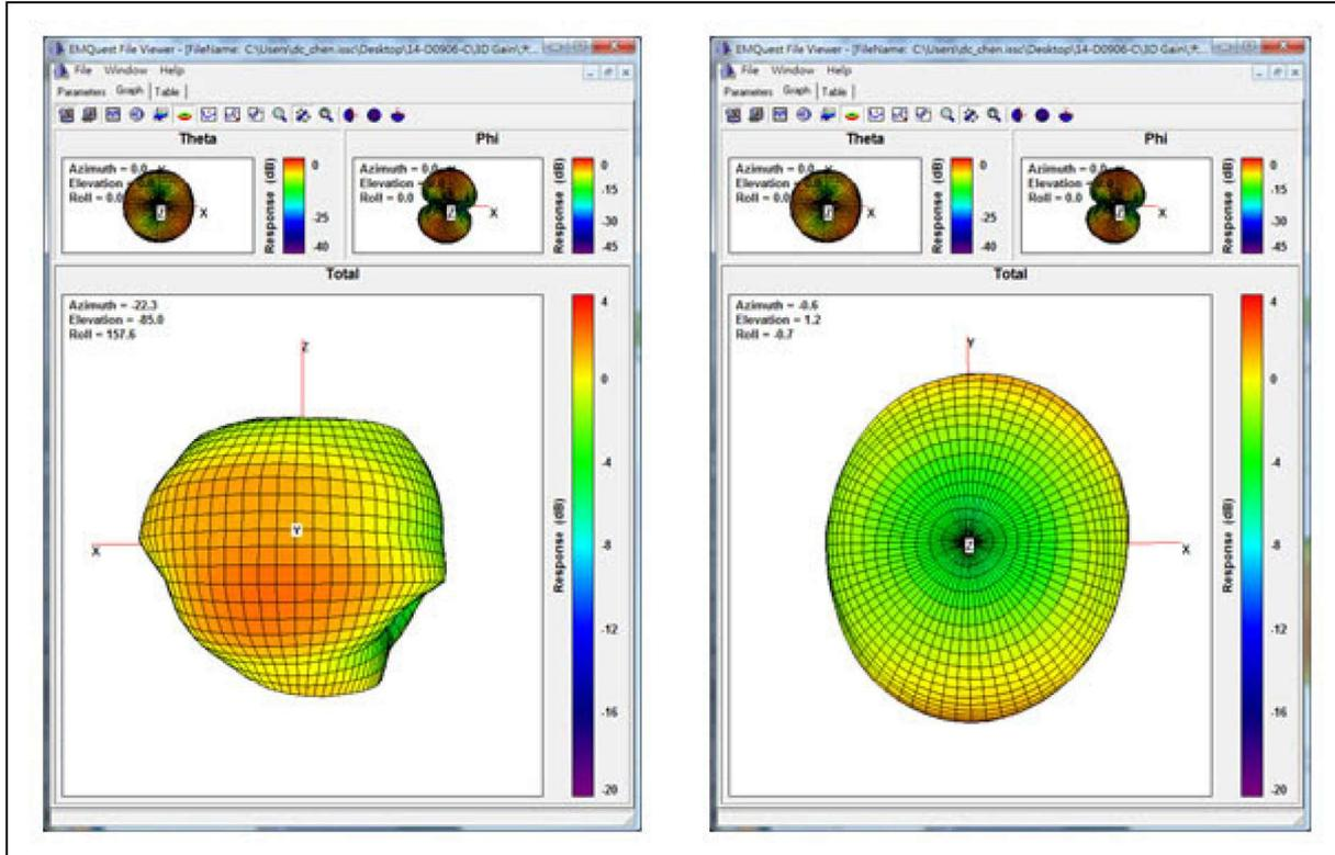
Table 6-1 provides the PCB Antenna characteristics of the BM62/64 module.
