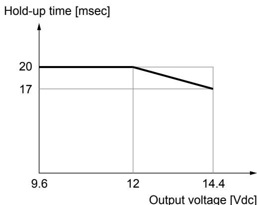
*Fig. 13: Hold-up time versus output voltage 12 V*
