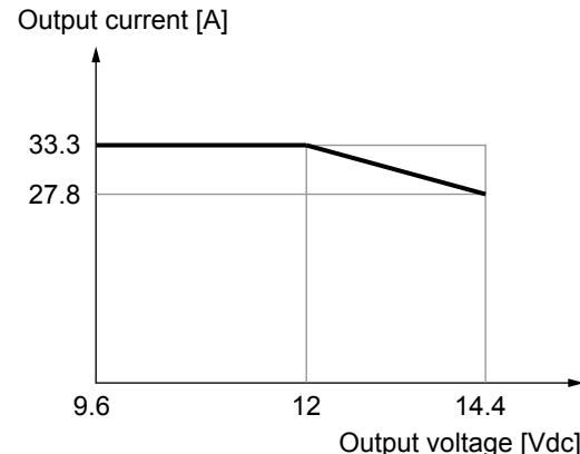
Fig. 10: Output current versus output voltage 12 V
