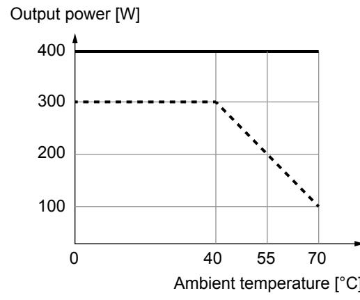
Fig. 8: Output power versus ambient temperature 24/48 V
