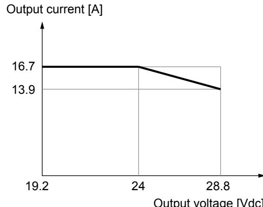
Fig. 11: Output current versus output voltage 24 V
