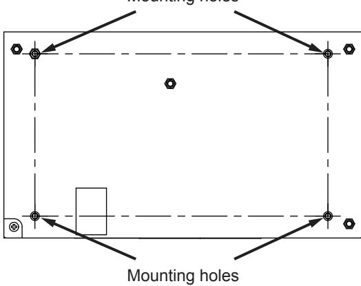
Fig. 5: Position of the mounting holes
