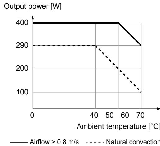
Fig. 7: Output power versus ambient temperature 12 V
