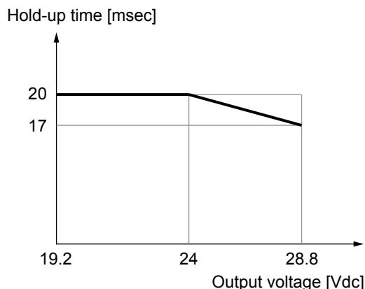
*Fig. 14: Hold-up time versus output voltage 24 V*
