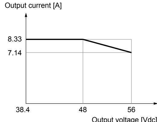
Fig. 12: Output current versus output voltage 48 V
