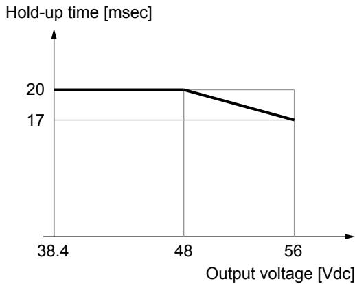
*Fig. 15: Hold-up time versus output voltage 48 V*
