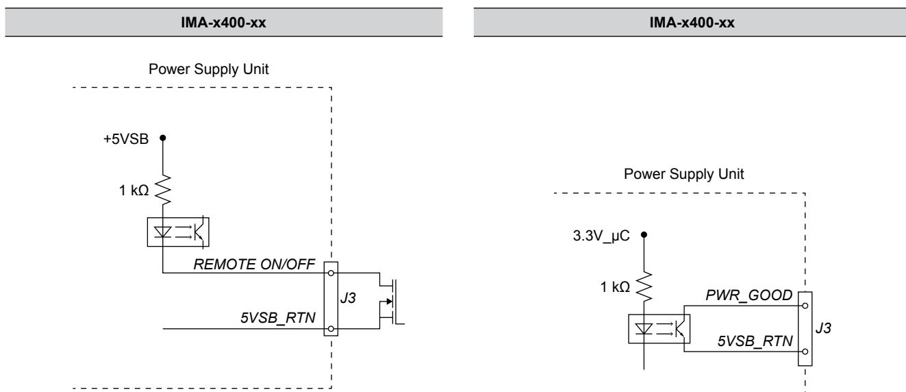
Fig. 20: Circuit diagram J3 Pin 10 (REMOTE ON/OFF)
