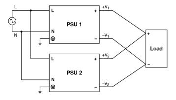
Fig. 4 Parallel Operation Connection Diagram
