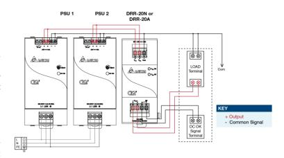
Fig. 3 Redundant Operation Connection Diagram
