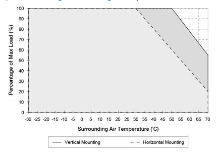
Fig. 1 De-rating for Vertical Mounting Orientation > 50°C de-rate power by 2.25% / °C
