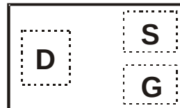
Top View Package Pin Configuration
