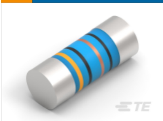
TE Model / Part #7-2176316-2 MELF SMA_A 68K 1% 50PPM 0207 1W
