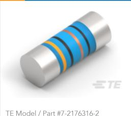
TE Model / Part #7-2176316-2 MELF SMA\_A 68K 1% 50PPM 0207 1W
