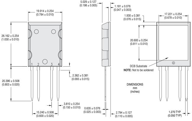
NOTE: Metallized external surface of DCB substrate maintains 2500V<sub>rms</sub> isolation to device internal structure and all external pins.
