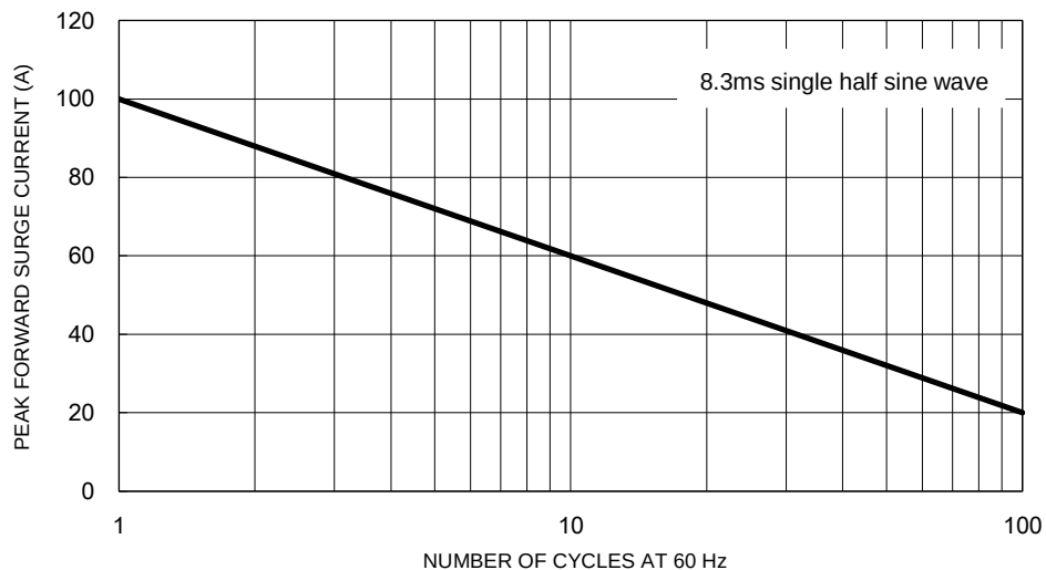
Fig.5 Maximum Non-Repetitive Forward Surge Current
