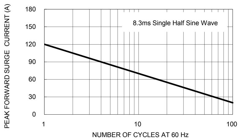
FIG. 2 MAXIMUM NON-REPETITIVE FORWARD SURGE CURRENT
